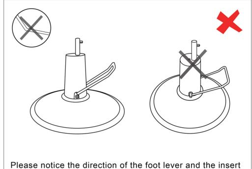
direction when installing the foot lever.
